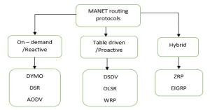
Figure 1: Routing protocols in Mobile ad-hoc network [1]
