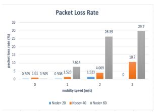
Figure 9: Packet loss rate at different number of speed and nodes
